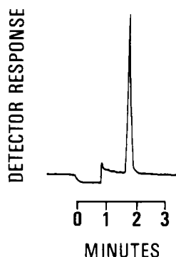
Figure 1. Sample chromatogram equivalent to 0.93 ng of NDPA.
